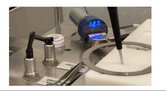
1.2.4. Mount the ring on the wafer and finger-tight the screws in a star pattern using the screwdriver
