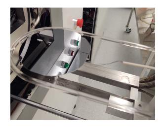
4.2 – Ensure the thermocouple is in contact with the back of the wafer.
